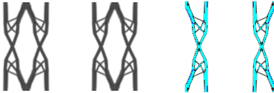
Figure 14: Stress-constrained optimized topology with continuation on stress limits (pseudo-Lagrangian cost function, SigTorq ) on the left. Normalized \sigma_{VM} distribution on the right. PEEK, Col1 seed geometry, V = 0.147 , \sigma_{VM,max} = 32 MPa
