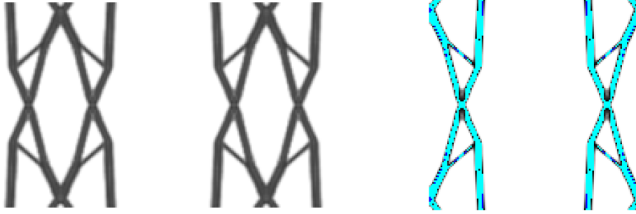
Figure 13: Stress-constrained optimized topology with continuation on volume, compliance and stress limits ( Cont ), on left. Normalized \sigma_{VM} distribution on right. PEEK, Col1 seed geometry, V = 0.13 , \sigma_{VM,max} = 32 MPa
