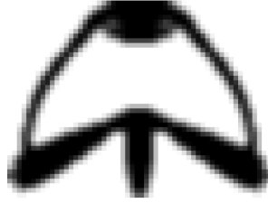
Figure 12: Optimized material layout for the unit cell of a bi-stable stent
