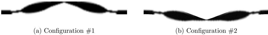
Figure 5: Optimized material layout for the bi-stable beam structure
