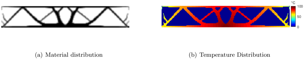
Figure 5: Optimized topology for the single material domain with combined thermoelastic objective, f_{obj} = 0.1290 , compliance= 14.21N·m, T_{ave} = 76.13^\circ\text{C}
